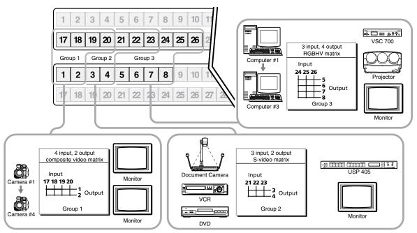
Figure 3-29 — I/O grouping of incompatible video formats
